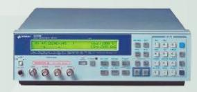
Surface & Volume Resistivity Tester Range 109 to 1016 Ohm/Ohm-cm
