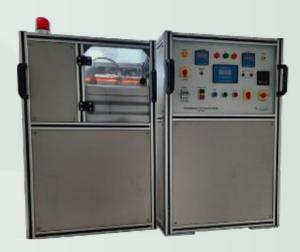
Programmable Dielectric Strength Tester up to 50 KV
